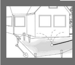
Permeable pavement allows water runoff to infiltrate through the soil and prevents most pollutants from reaching the storm drain system.
